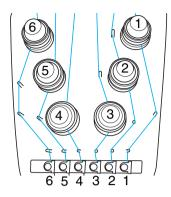
Pass the thread through the hole in the number 1 upper thread guide.
